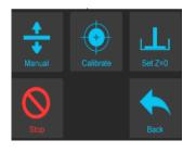
The manual page, also allows you to manually move the printer to the home (physical zero) position.
